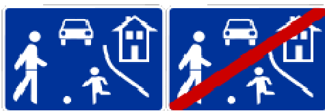
Sign 325 and 326 Begin and end of traffic calmed zones
